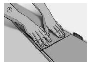
The remaining boards of the first row must be clicked in from above at the head ends into the previous boards. Pressure applied briefly to the side joint clicks in the board into the adjacent board. It is important to ensure that the first row is straight and exactly parallel to the wall. Cut the last board of the first row to size, leaving an expansion gap of 1015 mm (3/8"-1/2") between the board and wall. Fit in the board and lay it flat.
