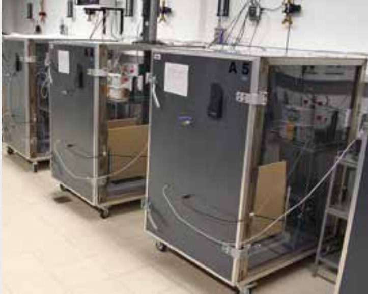
Test chambers with a volume of 1 m 3 at Fraunhofer Institute WKL.
